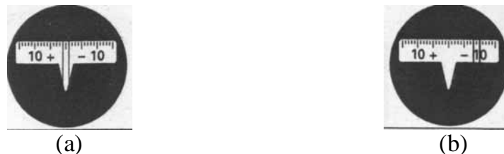
Figure 1: (a) Swing of the gyro mark of the scale. (b) Gyro mark at elongation-transit method. (Courtesy of Leica, Inc.)
