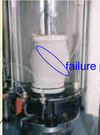
soil sample at failure
